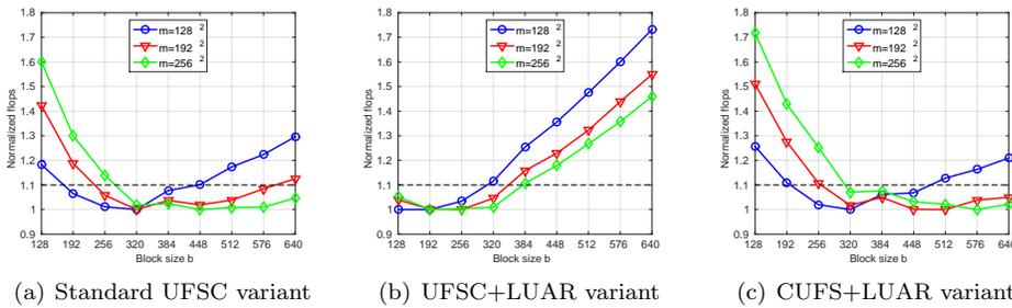
FIG. 13. *Normalized flops (i.e., the minimal is 1) for different block sizes  $b$  (Poisson problem,  $\varepsilon = 10^{-10}$ ). The block sizes under the dashed black line are those for which the number of operations is at most 10% greater than the minimal one.*
